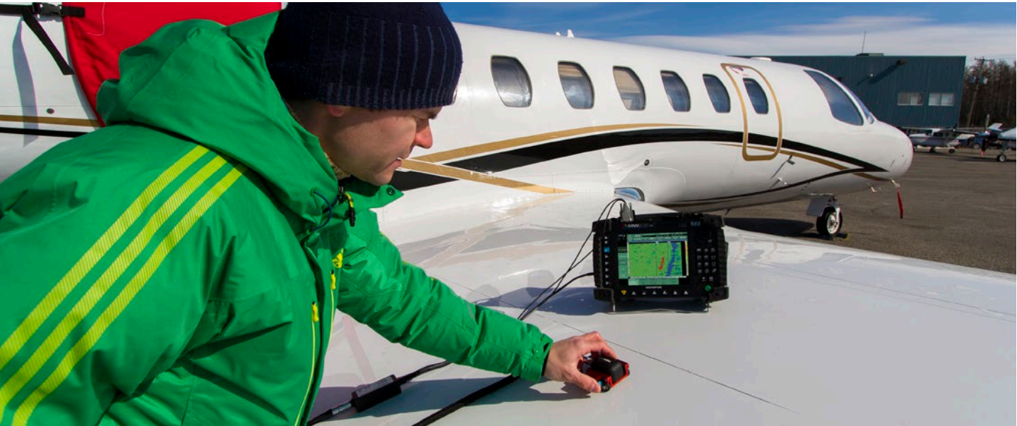
For maximum detection, the MXB software features 8-frequency scanning and amplitude and phase C-scan display.
