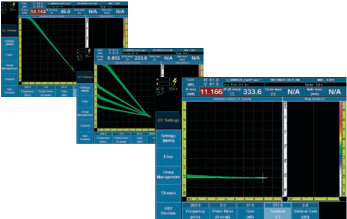
Adjust the phase angle in real time with the OmniScan knob. Gain, vertical gain, and null point (H/V) can also be adjusted the same way.
