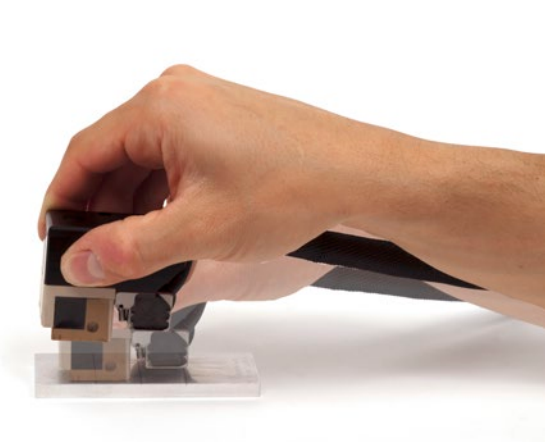
Generate live lift-off signals with an ECA probe – just like with a conventional ECT probe.
